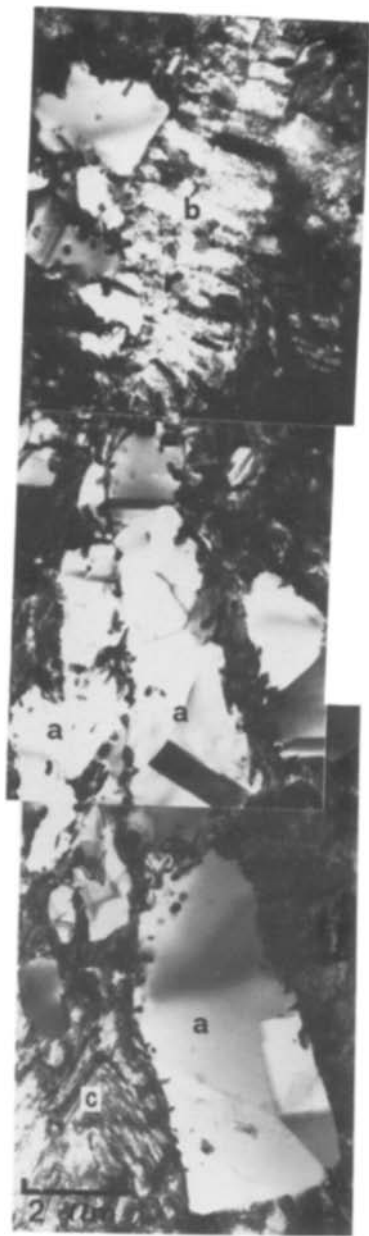
Figure 5 Microstructure of dynamically-compacted Inconel 718 after heat treatment at 800°C for 1 h. Powder particle boundaries show the beginnings of recrystallization (a), and the boundaries remain decorated with coarse carbide particles. The melted zones (b) formed during compaction do not recrystallize. Particle interiors still show the high dislocation and twin densities (c).
